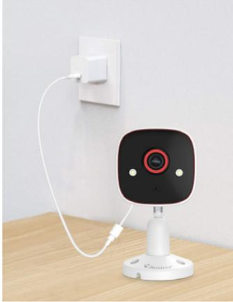
Power up using the Type-C power cable included in the box
