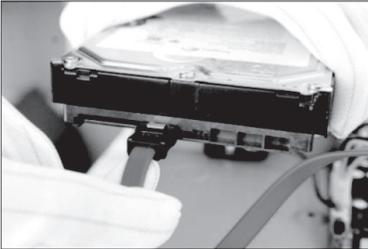
(3) Turn over the Device, and align the HDD to the four holes of bottom panel, and then fix the HDD with screws in the screw package.
