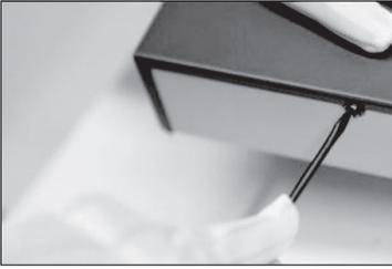
(1) Unscrew four fixing screws of the cover and remove the cover.
