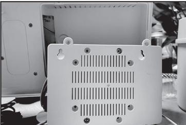
(3) Align the HDD to the four holes of back panel, and then fix the HDD with screws.
